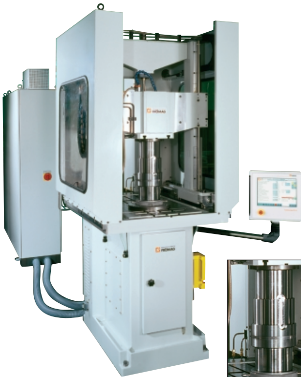
Rapida CNCE 100-750 with vertical and horizontal moveable centring and receiving unit
